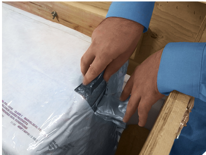
Figure 4-11. Exposing the Eye-bolt Holes
