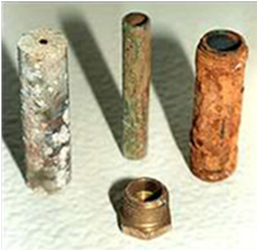
Untreated Water Circuit
