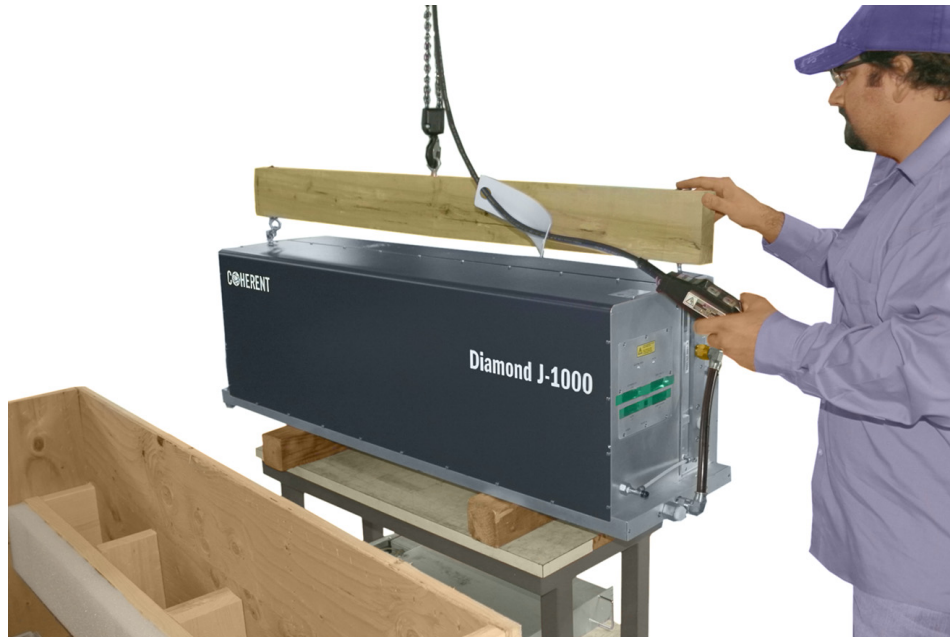
Figure 4-17. Place Laser System on Cart
