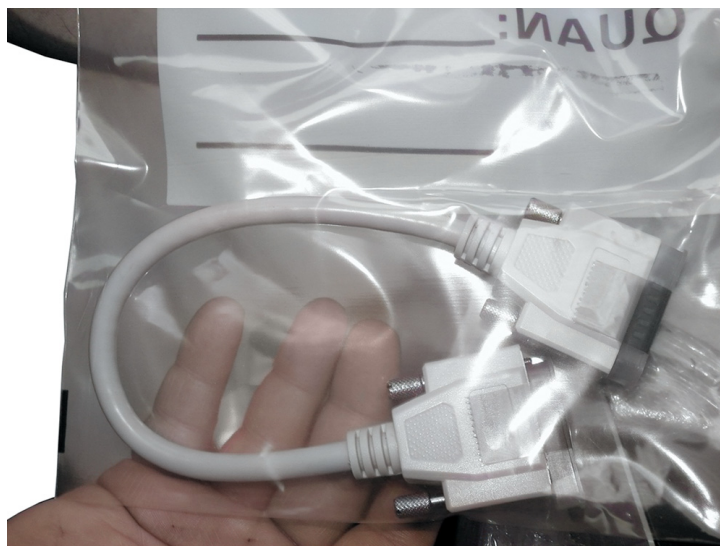
Figure 4-18. RF Power Module System Cable
