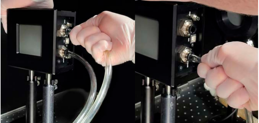
Figure 15. Attach Water Hoses Directly to Fittings on Sensor
