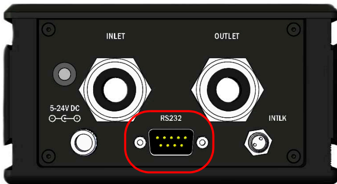
Figure 19. RS-232 Connector - RS-232 Model
