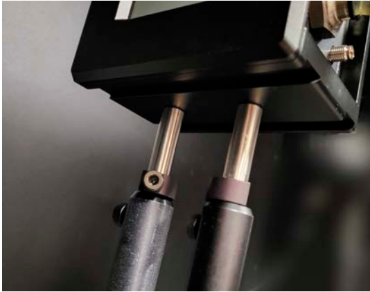
Figure 11. Direct Post Mount Setup Example
