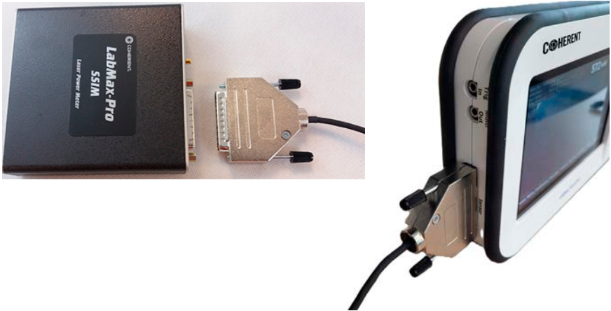
Figure 22. Connect Sensor to Meter with DB25 Cable
