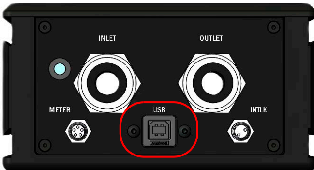
Figure 18. Sensor System USB Connector - USB Model
