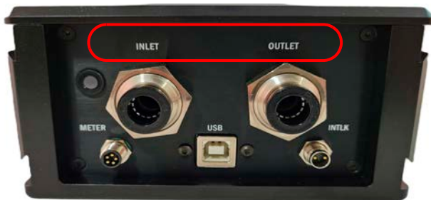
Figure 14. Water Inlet and Outlet Fitting Labels
