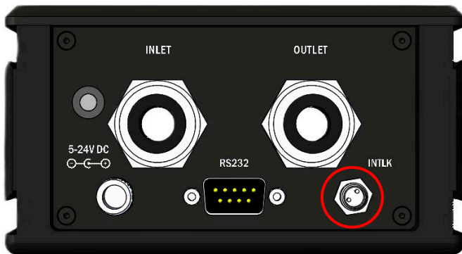
Figure 24. Interlock Connector (PM10K+ RS-232 Model)
