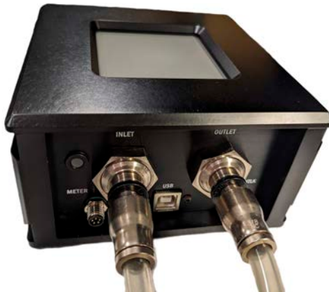
Figure 17. Water Hoses Installed With Step-down Fittings
