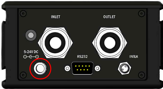
Figure 23. Power Connector - PM10K+ RS-232 Model
