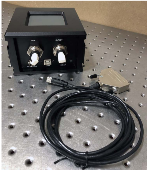
Figure 4-32. DB25 Cable for with USB+DB25 PM10K+ Configuration
