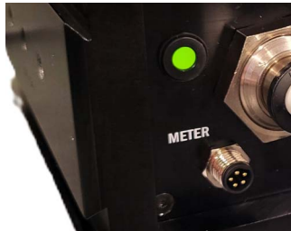
Figure 6-2. LED Status - Green at Correct Flow Level
