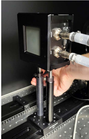
Figure 9-4. Loosen Mounts (PM10K+ example)
