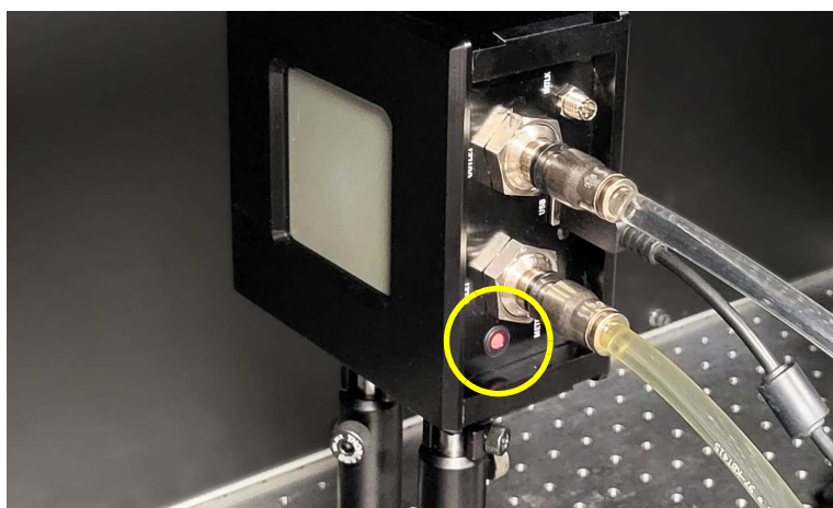
Figure 5-2. LED Indicator Light - Fault Condition Alarm (red)
