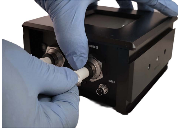
Figure 9-7. Remove Protective Plug Caps
