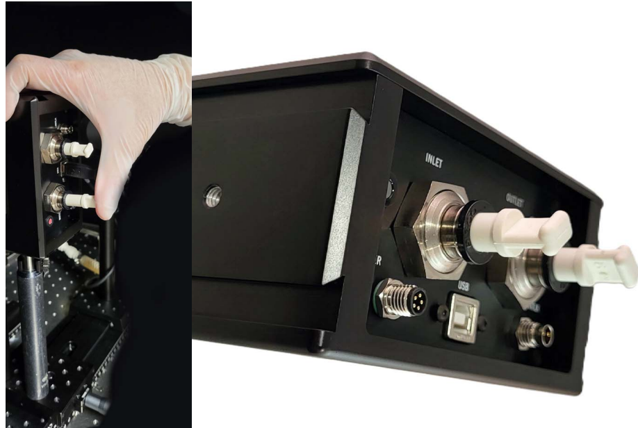
Figure 9-5. Water Cap Plugs Installed
