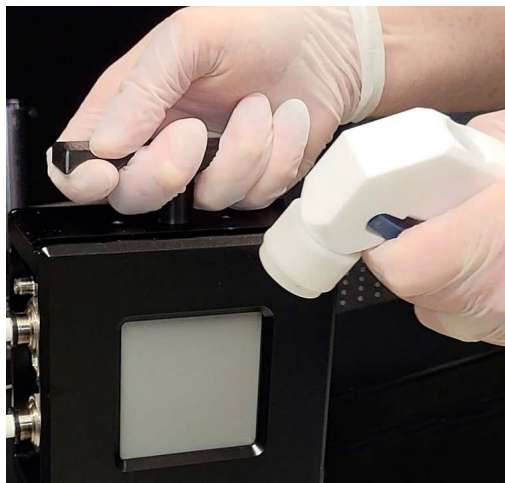
Figure 9-10. Clean with Clean Dry Air
