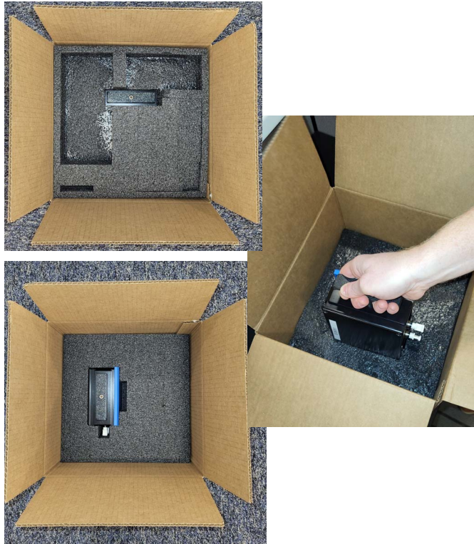
Figure 9-15. Set Sensor Into Bottom Foam Tray
