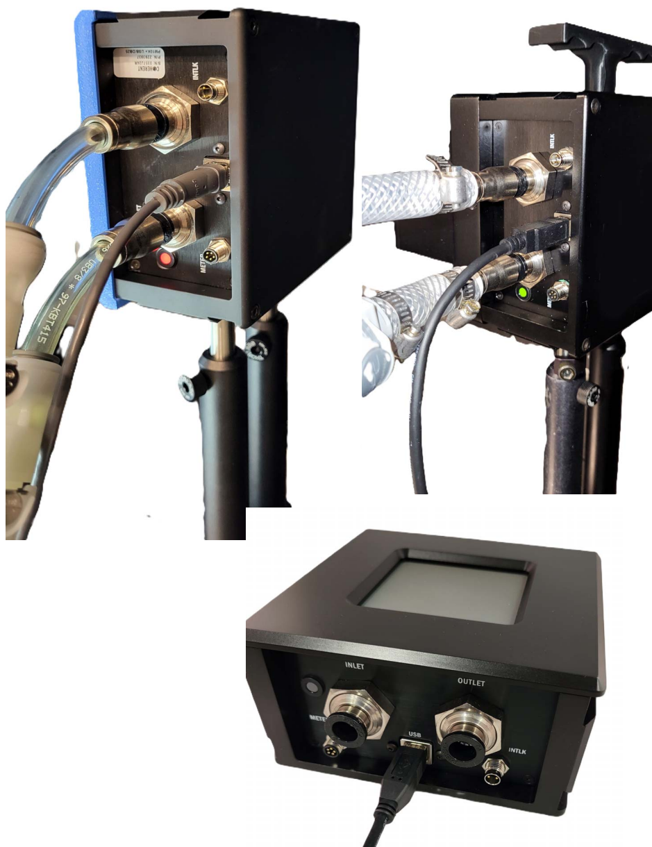
Figure 4-28. Attach USB Cable (PM10K+ Examples)
