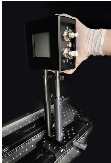
Figure 9-6. Remove Sensor from Mount (Post-mount setup)
