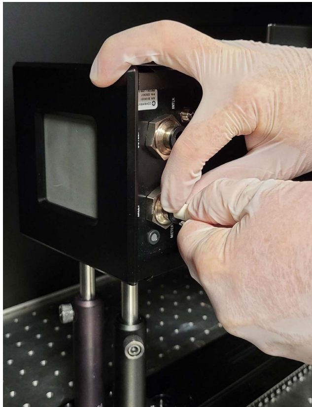
Figure 9-2. Remove Water Hoses from Sensor Fittings
