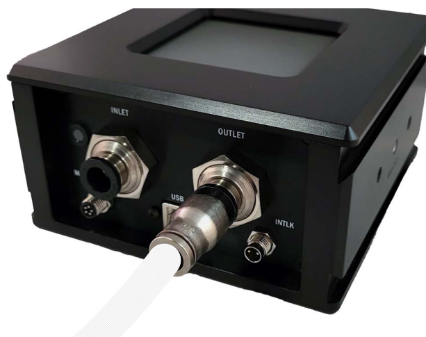
Figure 4-25. Insert Hose, with Adapter, into Fitting on Sensor
