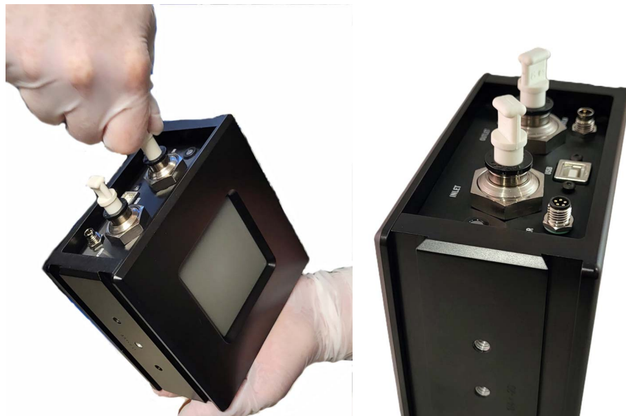
Figure 9-9. Reinstall Install Protective Plug Caps
