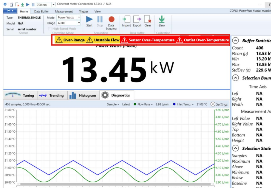
Figure 7-6. Measurement Panel - Warnings and Error Indicator Location
