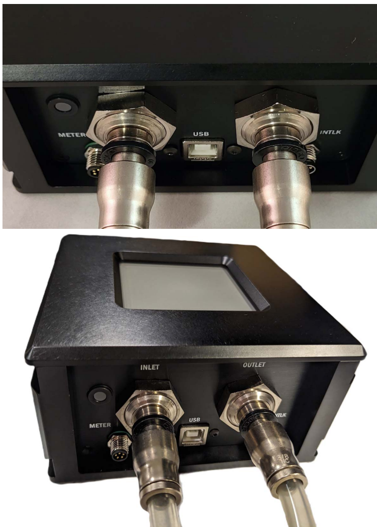
Figure 4-26. 3/8-in Hoses with Adapters Installed
